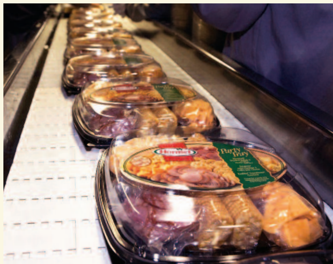
Converting the Hormel® party trays from a round to a square tray reduced material waste.
